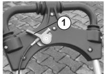
Control drive speed and direction of travel with the handle (1).
