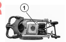
Fit the crane hook into the lifting ring (1) and lift the machine onto the desired means of transport.
